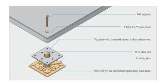
The system floor pedestal type RSP201 M18 made from galvanized steel in combination with threaded bolt base and steel flat-head is used as a perimeter pedestal for low-profile raised access floor system. The system floor pedestals are entirely made by Rhino, from the production design to the including galvanization.
