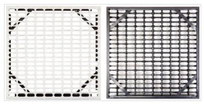
The raised access floor system RhinoROC® 50% airflow perforated panel is perfectly suited for the use in technical rooms, server rooms and data centers. It consists of a welded tube frame structure with powder-coated surface and perforated covering sheet with elliptical holes. The substructure consists of height-adjustable zinc-coated steel pedestals from our own production which form the necessary cavity for installations and gaskets for sound decoupling.
