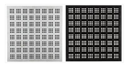
The raised access floor system RhinoROC® 25% airflow perforated panel is perfectly suited for the use in technical rooms, server rooms and data centers. It consists of a welded tube frame structure with powder-coated surface and perforated covering sheet with round holes. The substructure consists of height-adjustable zinc-coated steel pedestals from our own production which form the necessary cavity for installations and gaskets for sound decoupling.
